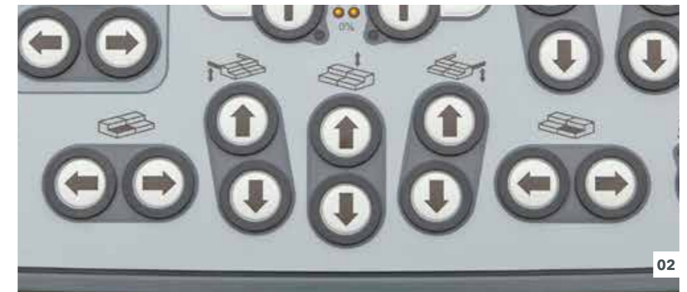
01 Precompaction performance 02 Screed settings
