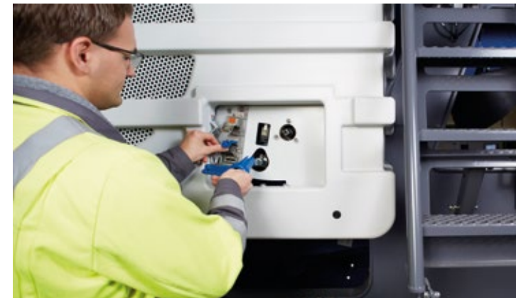
> Insert control element in the enable station; the rotor is safely locked and the key is enabled for further steps.
