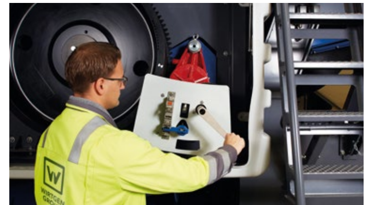
> The rotor is turned safely with the crank and moved into the optimum position for rotor ledge replacement.
