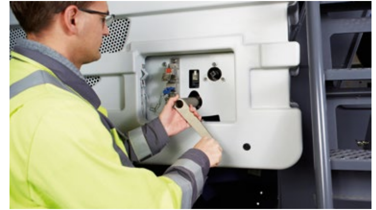
> The rotor locking and turning device is enabled and can be moved with a crank.
