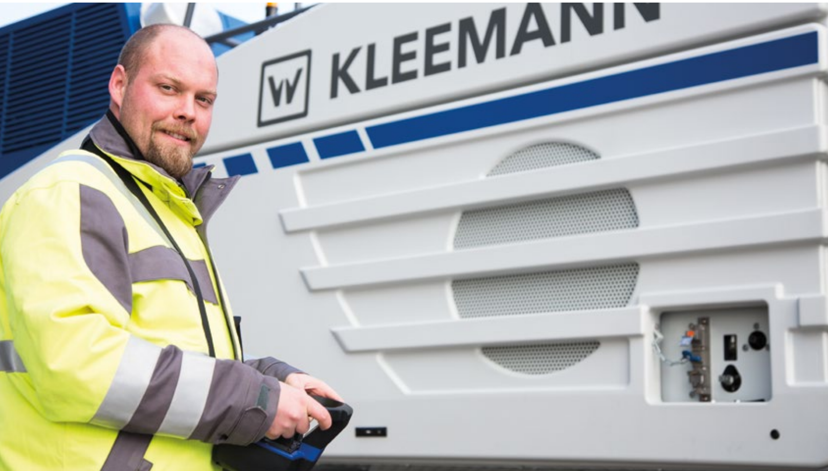
> Insert control element in the enable station; the rotor is safely locked and the key is enabled for further steps.
