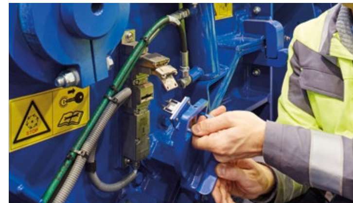
> The crusher housing is opened with a special key. The key cannot be removed once opened and material can be cleared safely.
