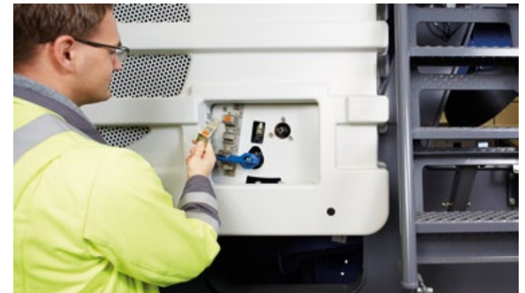
> If keys are removed, the rotor remains safely locked.
