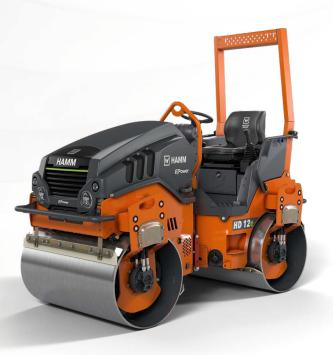
Tandem rollers Series HD CompactLine Tandem roller with two vibrating roller drums
