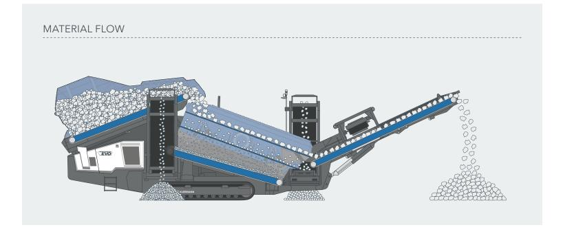
With its proportionally controlled running gear, the plants for coarse screening can be moved quickly and precisely, whether from the low-loader to the application site or within the work site. The side discharge conveyors can be folded without the need to assemble or disassemble any components, thereby reducing set-up times.
