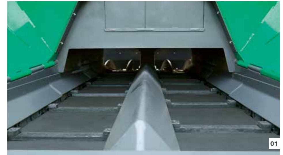
01 Proportional control and continuous monitoring of augers guarantee a constant head of mix in front of the screed in line with current requirements.
