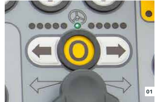
01 For long curves with a constant radius, the desired steering angle can be preselected using arrow keys.
