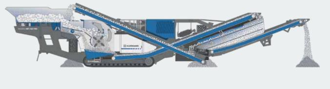
The MOBIREX MR 130(i) PRO excels with outstanding product quality and very high product output. The Continuous Feed System (CFS) guarantees continuous crusher utilisation. Thanks to the fully hydraulic crusher gap adjustment, machine parameters can be adapted quickly to the application. The overload system ensures effective
