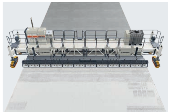
Applying a broom finish and spraying in longitudinal direction broadens the range of options to produce different surface textures.
