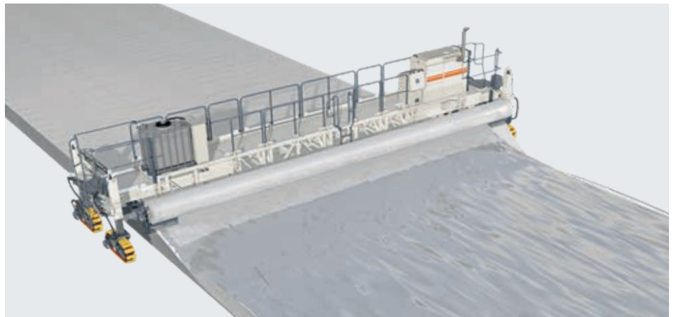
Film unwinder for effective protection of the concrete in case of rain.
