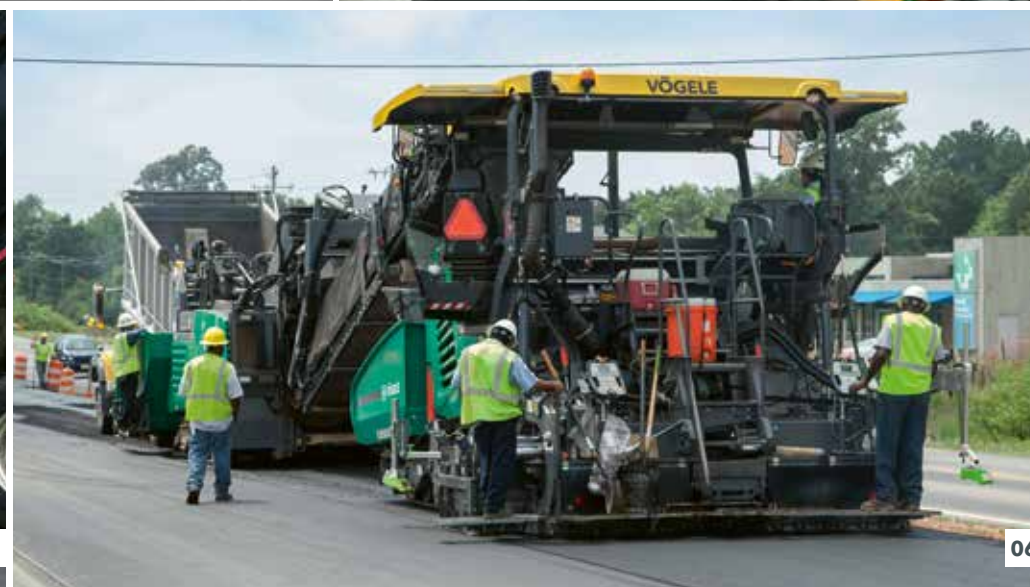
04 ErgoPlus 3 with numerous additional ergonomic and functional advantages. 05 Optimum feeding with mix thanks to the large material hopper. 06 The right screed for every application. The paver can be combined with the VF 600, VR 600 and AB 600 Extending Screeds.
