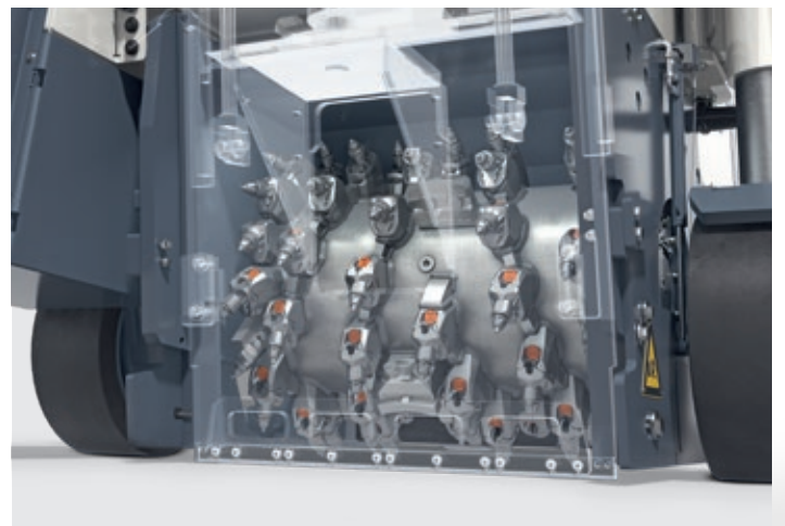
Intelligent milling drum design.
