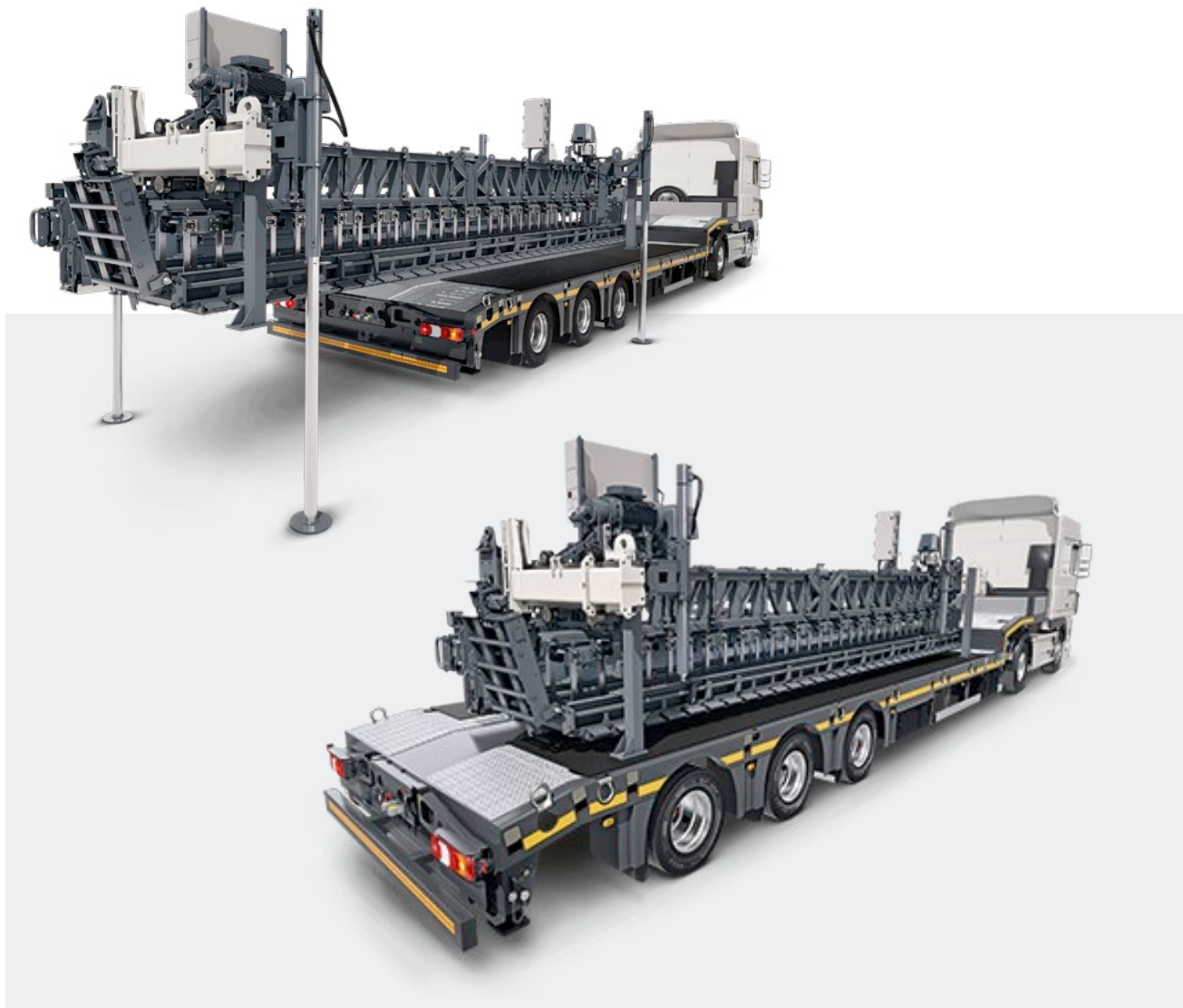
Self-loading dowel bar inserter.
