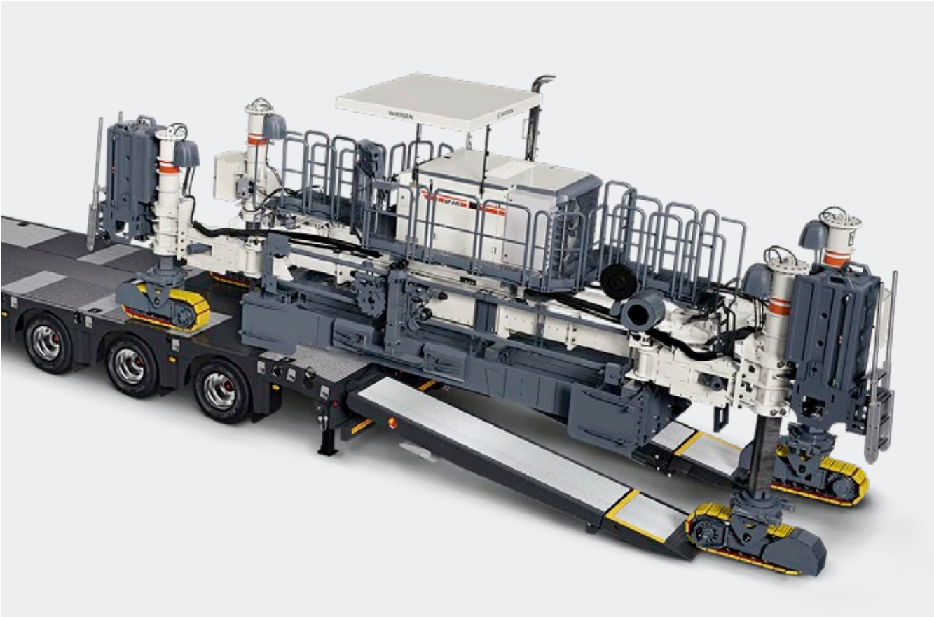
Hydraulic swing legs for easy transportation and a high degree of flexibility on construction sites.
