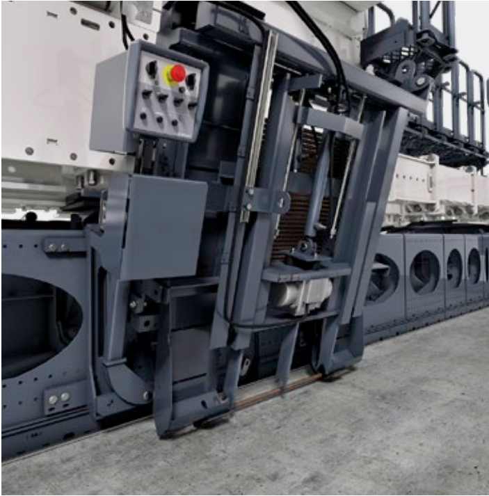
Longitudinal tie-bar inserter with control unit.
