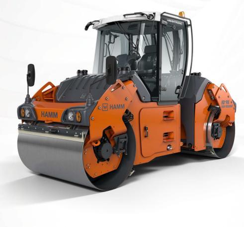
Tandem rollers Series HD+ Tandem roller with two vibrating roller d H303
