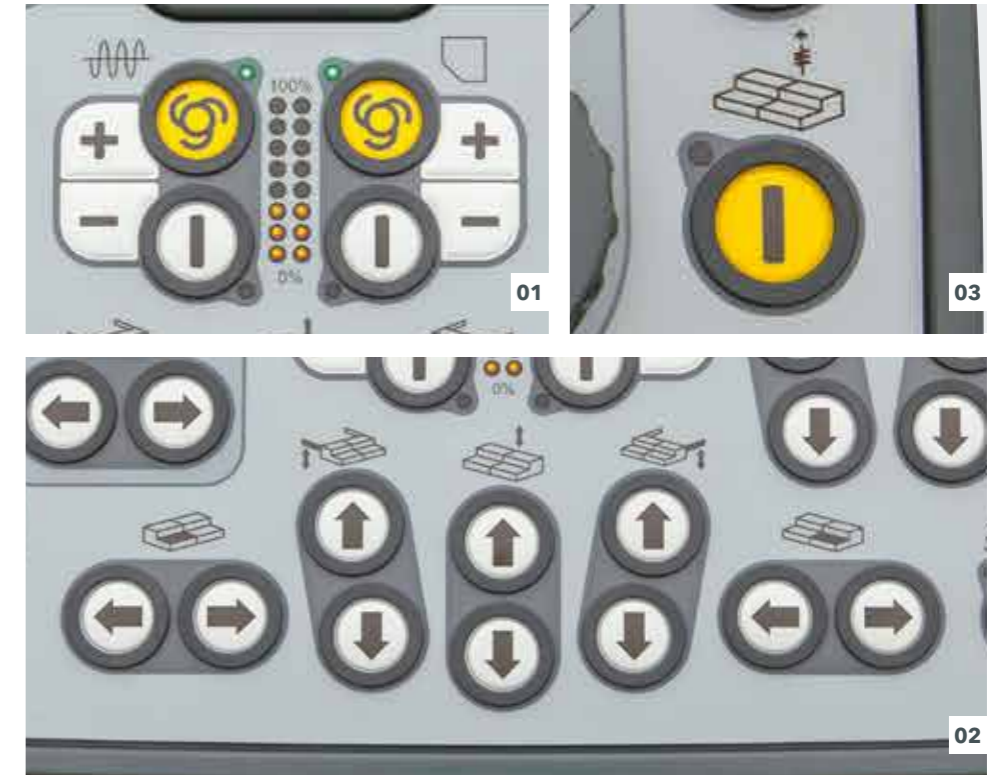
01 Precompaction performance 02 Screed settings 03 Screed Assist (option)
