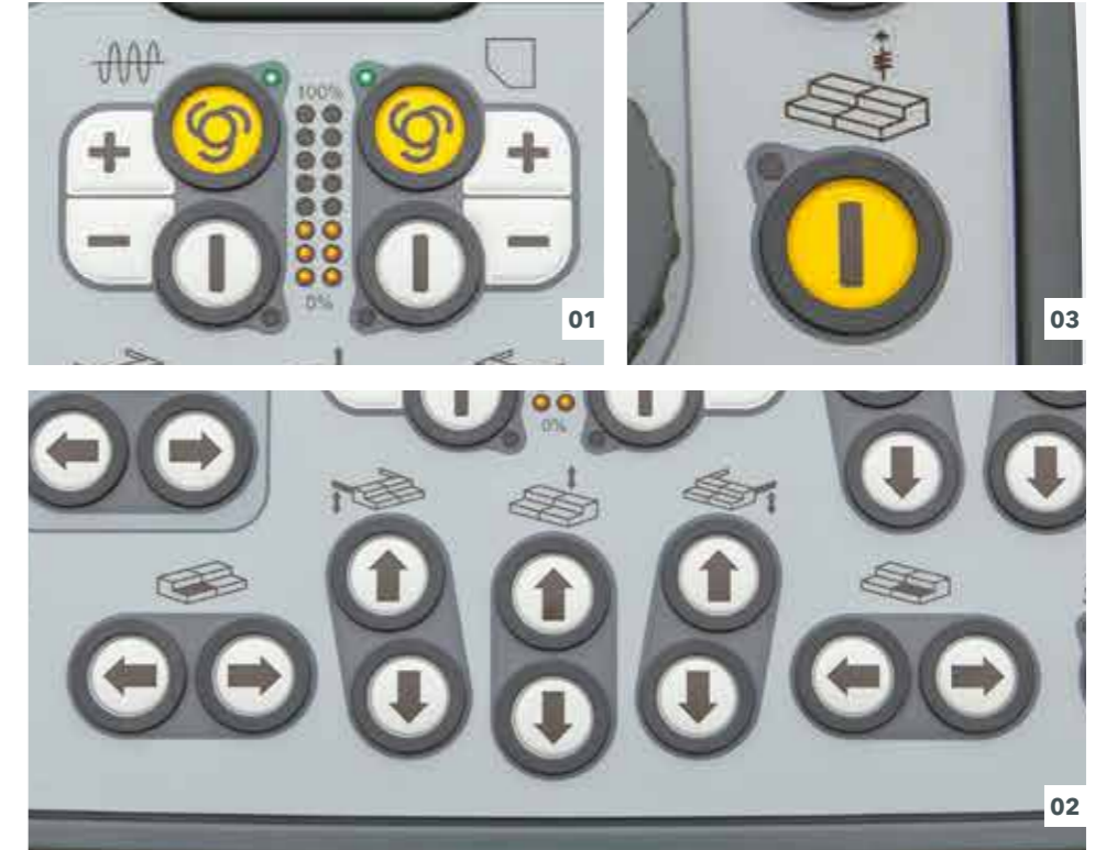
01 Precompaction performance 02 Screed settings 03 Screed Assist (option)
