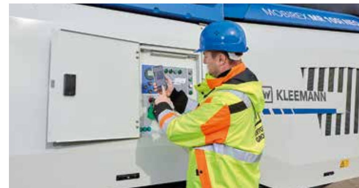
1. Connect the MR 100i NEO with SPECTIVE CONNECT by simply scanning the access data from the machine's display.
