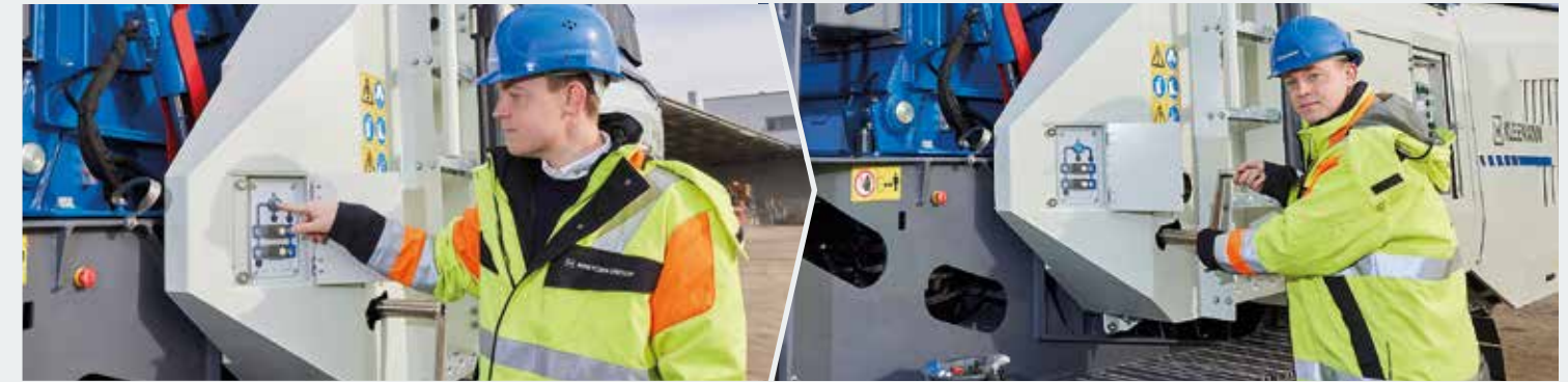
> The rotor locking and turning device is released at the touch of a button... ...and engaged by hand crank.
