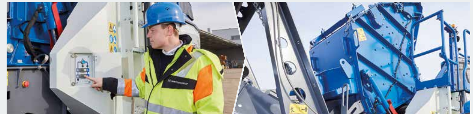
> Automatic opening of the crusher housing when the button is held down... ...until the crusher opens completely. The mechanical safety catch also engages.
