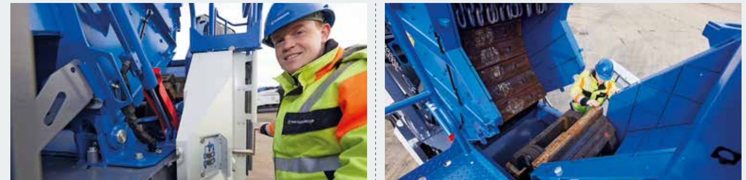
> The rotor is moved into position for wear check or rotor ledge replacement. The crusher is opened completely for best possible access for service and maintenance from both sides. Rotor ledge replacement takes place easily from above.
