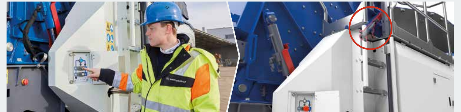
> The crusher is unlocked at the push of a button... ...and the wedges for locking the crusher housing are pulled hydraulically.
