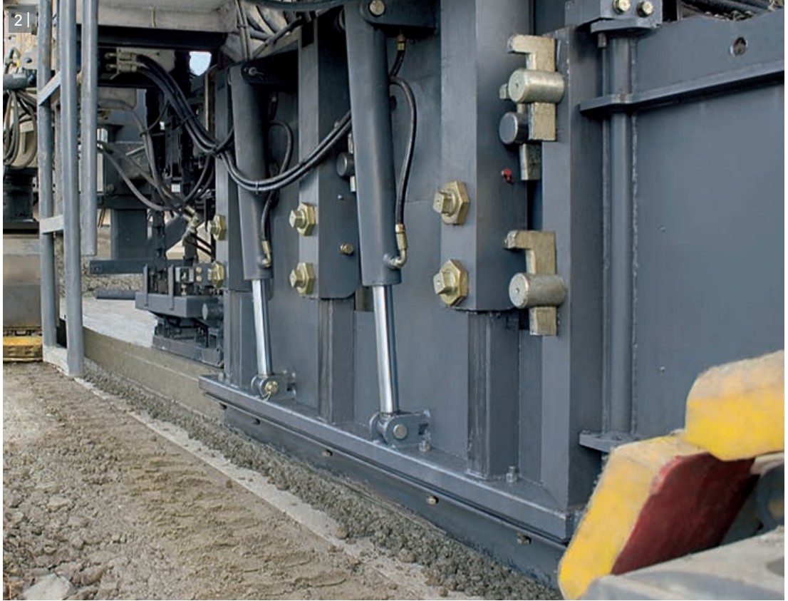
2 | Hydraulically adjustable side plates produce clean edges.
