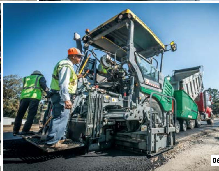
04 ErgoPlus 3 with numerous additional ergonomic and functional advantages. 05 Optimum feeding with mix thanks to the large material hopper. 06 The right screed for every application. The paver can be combined with the VF 500 Extending Screed.
